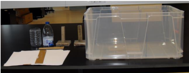
Figure 1. Material available: plastic container, wooden plates for soil compaction and paper (reinforcements).
