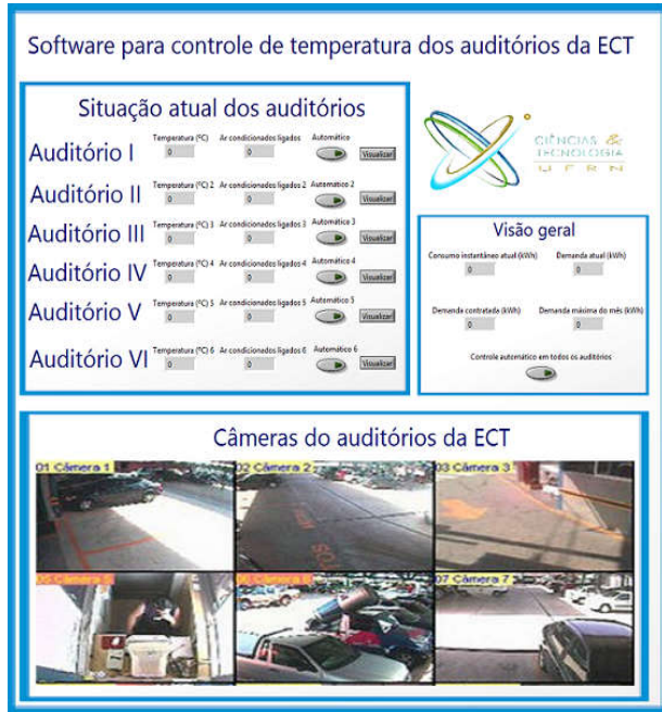
Fig. 2. Interface for monitoring and controlling of ECT's cooling system – general view.
