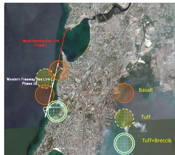
Figure 3. Areas with different rock types along proposed bridge alignment
