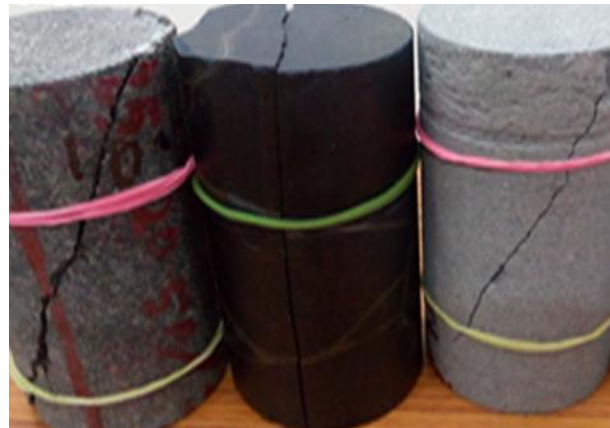
Figure 7. Typical failure patterns under uniaxial compression tests.
