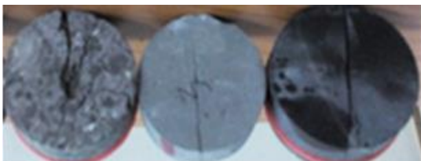
Figure 6. Typical failure patter under indirect tensile test.
