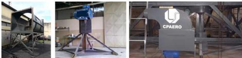
Figure 11: Engine support (left); drive system section (middle) and Cooling system to extract hot air inside the engine cavity (right).
