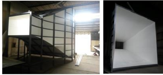
Figure 10: Contraction part - details.
