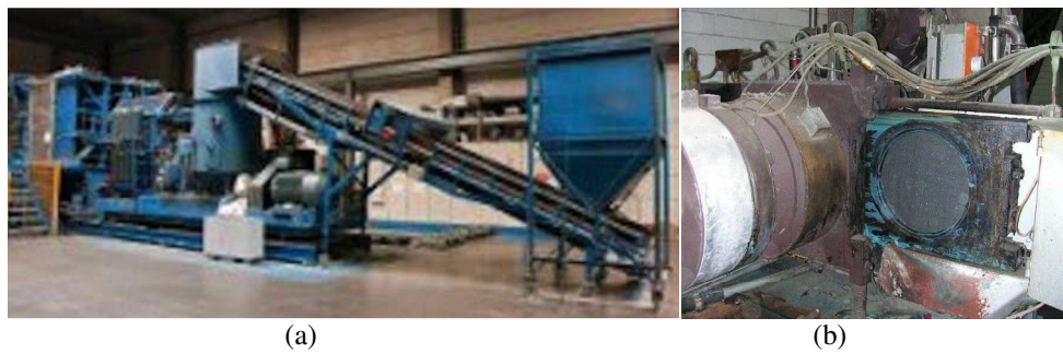
Figure 5: (a) the plastic sequins into the extruder; (b) detail of the heater bands (REZENDE JÚNIOR)
