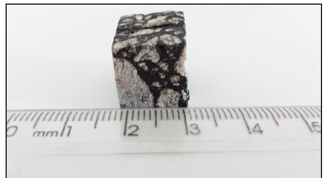
Figure 5: Asphalt concrete test sample with dimensions close to one centimeter.
