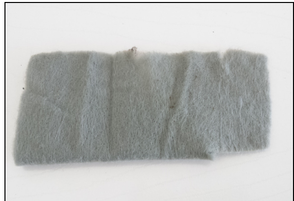
Figure 1: Type of Geotextile used to reinforce asphalt concrete specimens.
