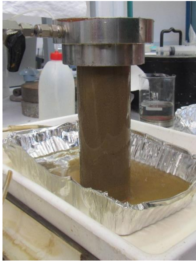
Figure 1. Consolidation test specimen preparation by slurry deposition
