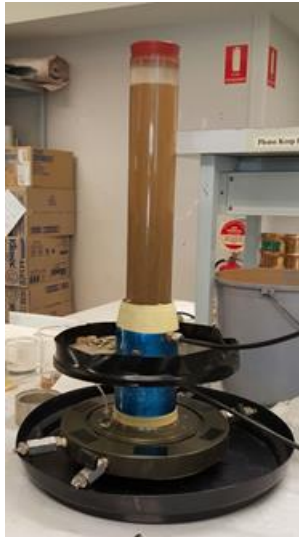
Figure 2. Triaxial test specimen preparation by slurry deposition
