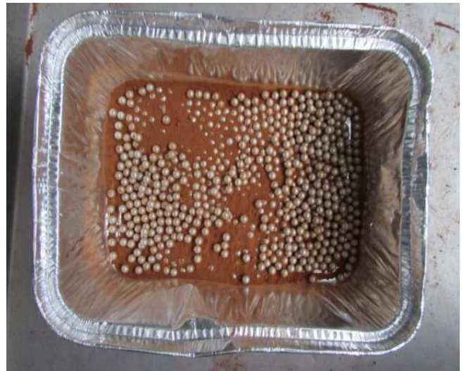
Figure 3. Mixture residual soil-steel spheres
