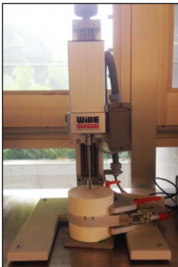
Figura 3. Vane shear test.
