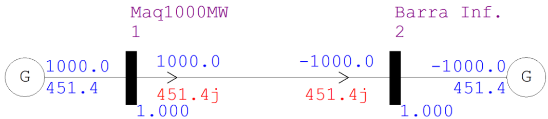
Figure 1: Infinite bus circuit designed using ANATEM software.
