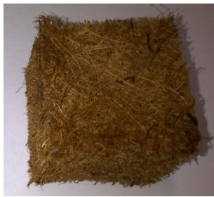
Figure 2: Coconut fiber specimen measuring 50x50x45 mm 3
