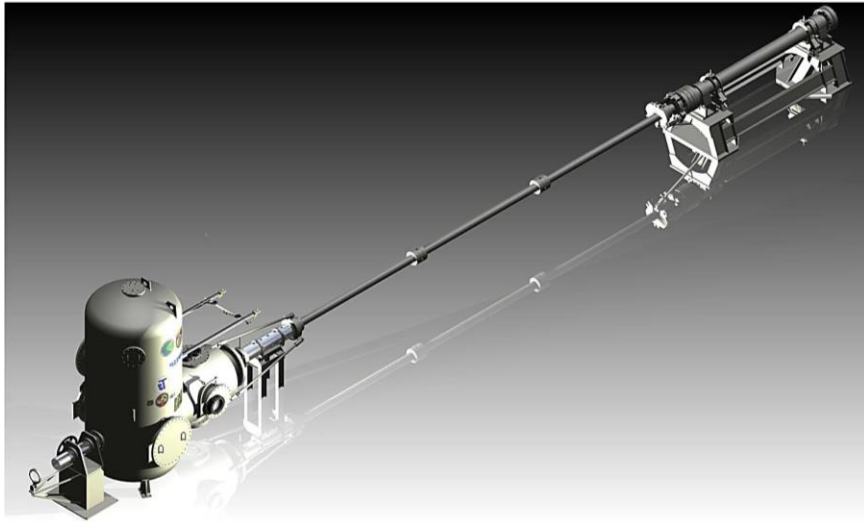
Figure 2. T3 0.61-m. nozzle exit diameter Hypersonic Shock Tunnel.
