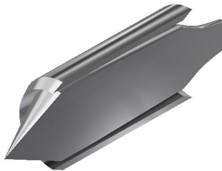
Figure 4: Geometry of the Brazilian academic unpowered axisymmetric scramjet.
