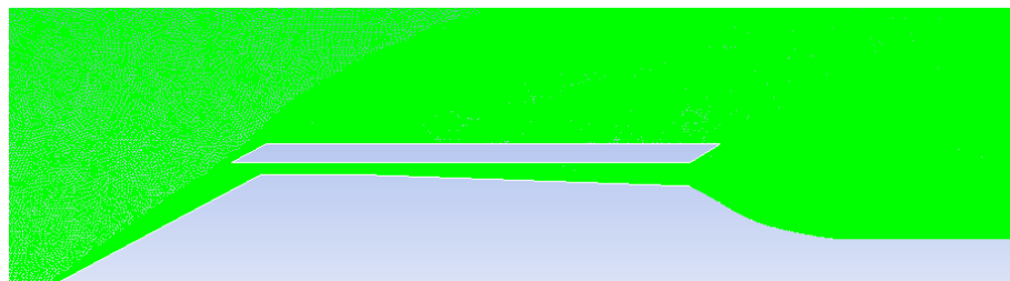
Figure 7: Academic scramjet computational grid. Details of the high grid resolution at the inlet, combustor and outlet.
