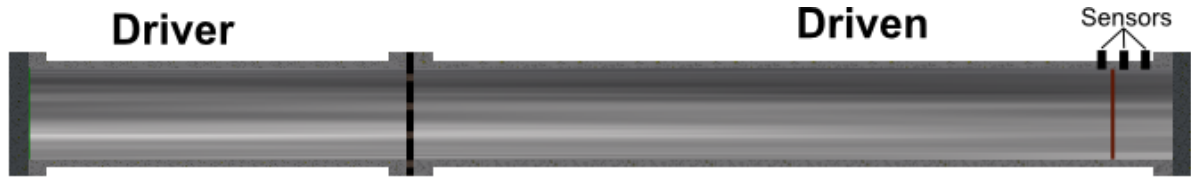
Figure 7 – Operating diagram of a shock tube with sensors installed at the end of Driven
