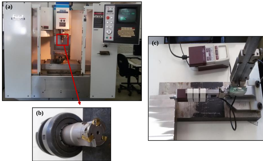
Figure 1. FADAL VMC (a), Rectangular inserts (b), Mitutoyo portable roughness (c).
