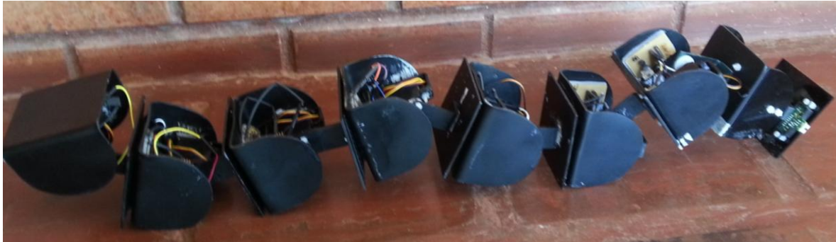
Figure 2. Sigma Lily in pitch-pitch configuration on flat ground.
