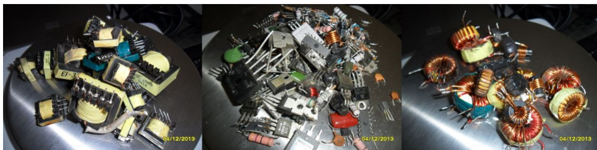
Figure 4: Electronic components removed from PCB.
