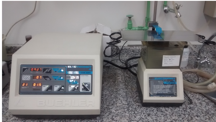
Figure 3: Electrolytic polisher for the creation of a controlled mass loss with progressive depth.
