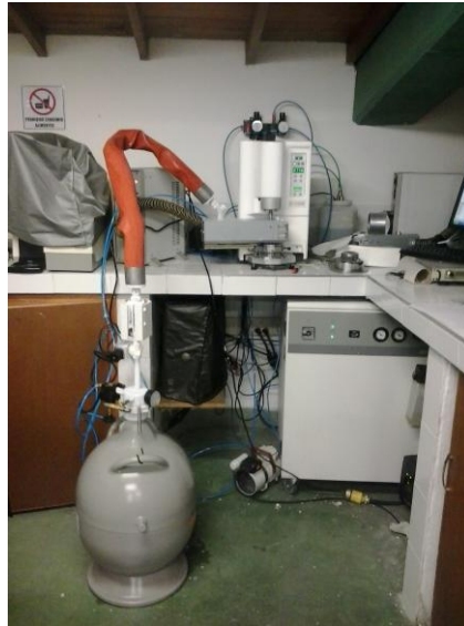
Figure 1. Rotational rheometer Bohlin C-VOR with cooling / heating ETC fed by liquid nitrogen for temperature control
