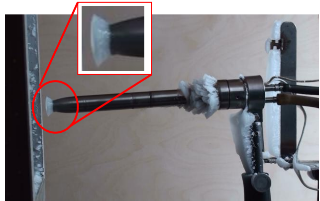
Figure 6.b. Ice shape over Pitot probe as obtained in the TsAIG Climatic Icing Wind Tunnel, Russia (Prof. Ivan Egorov, Head of TsAGI research department, private communication)
