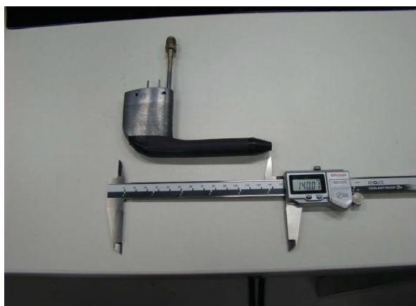
Figure 1.a. Pitot probe PH-510 used for illustration of the proposed thermal model
