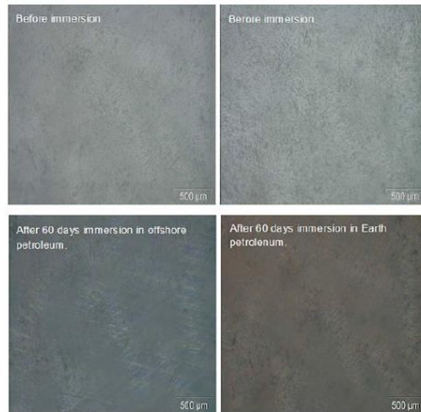
Figure 5 – Optical Microscopy (x100) of sample D (with 20% of \text{TiO}_2 ) before and after immersion in earth and offshore crude petroleum.
