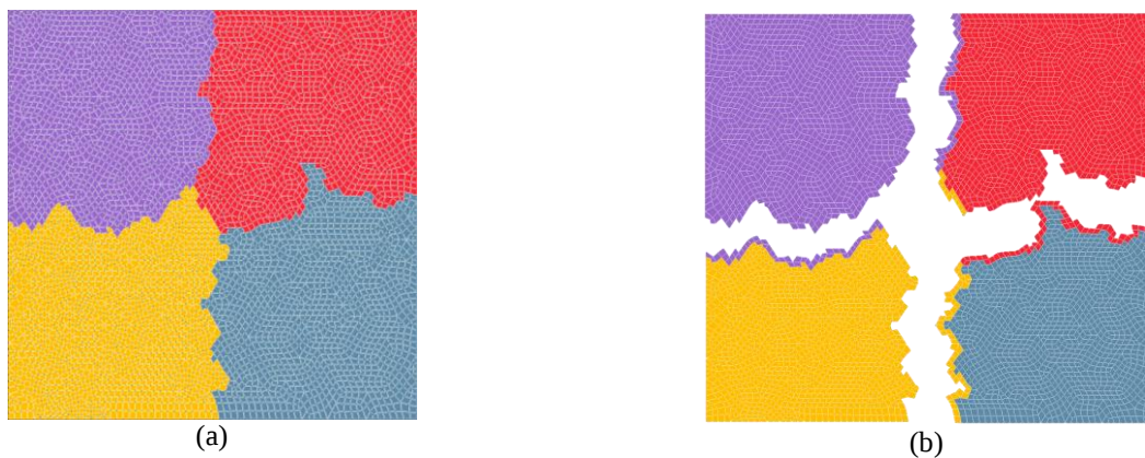
Figure 2. Two-dimensional grid division for parallel simulation. (a) – Grid partition (b) – Grid partition and ghost layers.
