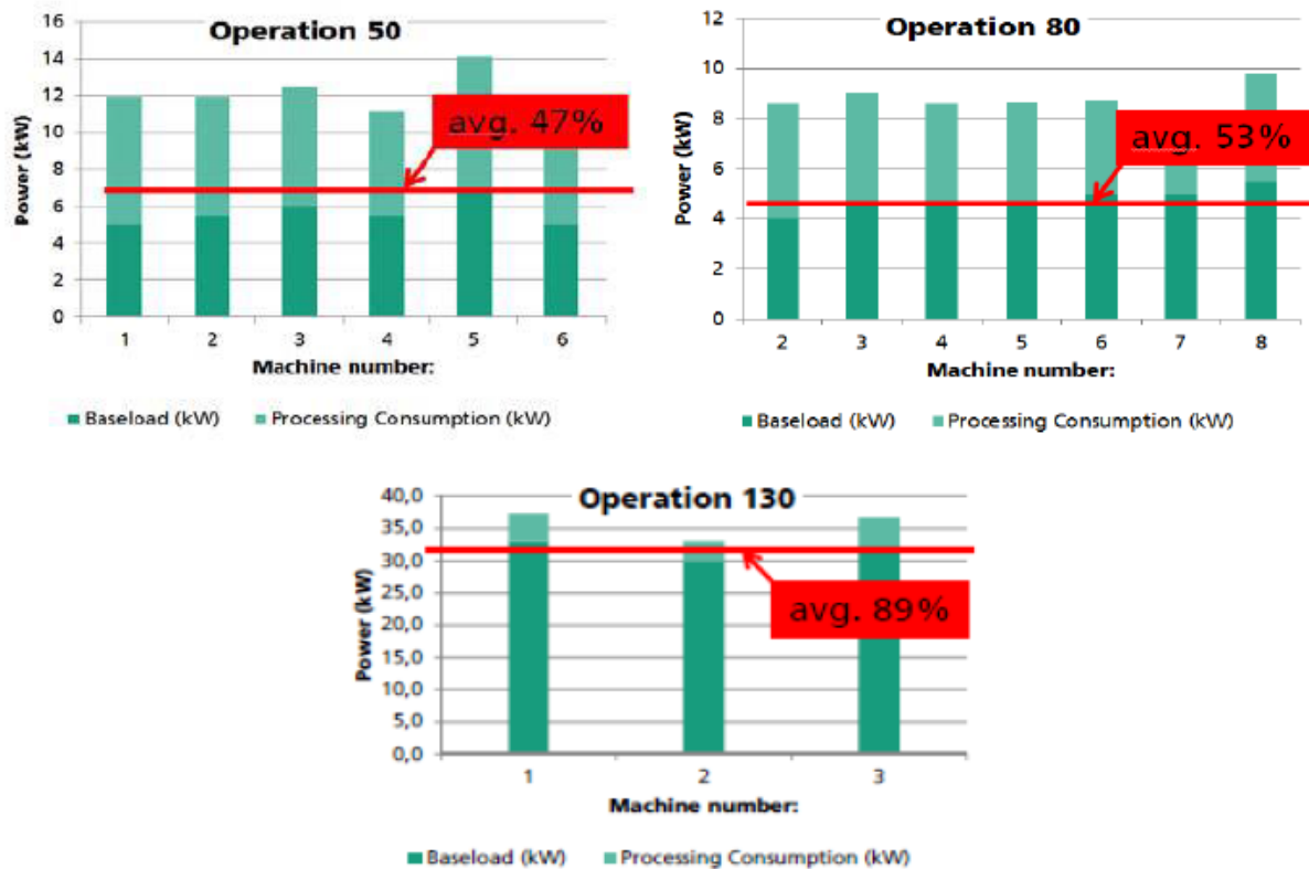
Figure 7. Base load energy consumption in comparison with the direct processing-related consumption for operation 50 and 80 (Cylinder block Line) and OP130 (Crankshaft Line).
