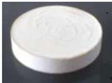
Fig. 3 - The sample test body 03 MF sintered at 1.400 °C.
