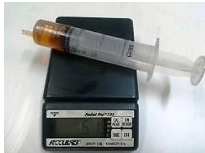
Figure 3: Metal Conditioner quantity to add on bearing. Source: Author.
