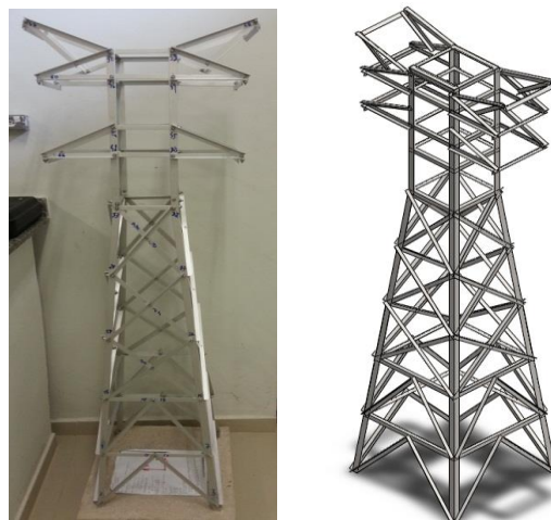
Figure 1. Constructed tower with the CAD platform projected model.
