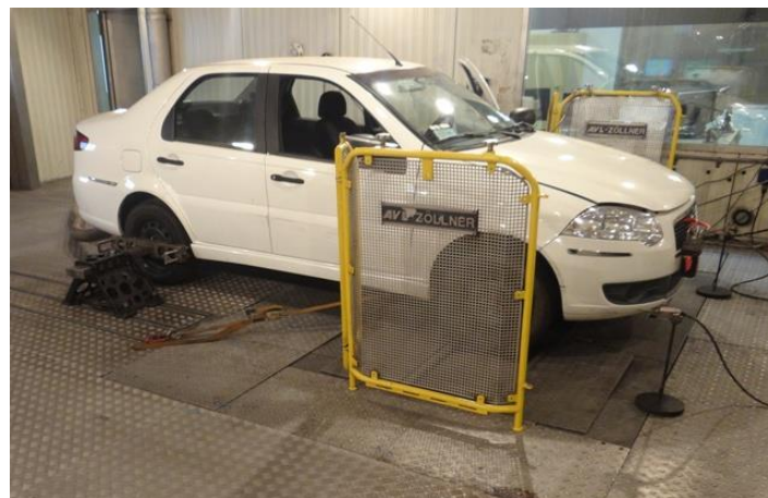
Figure 2. Vehicle mounted on chassis dynamometer for proof of consumption.
