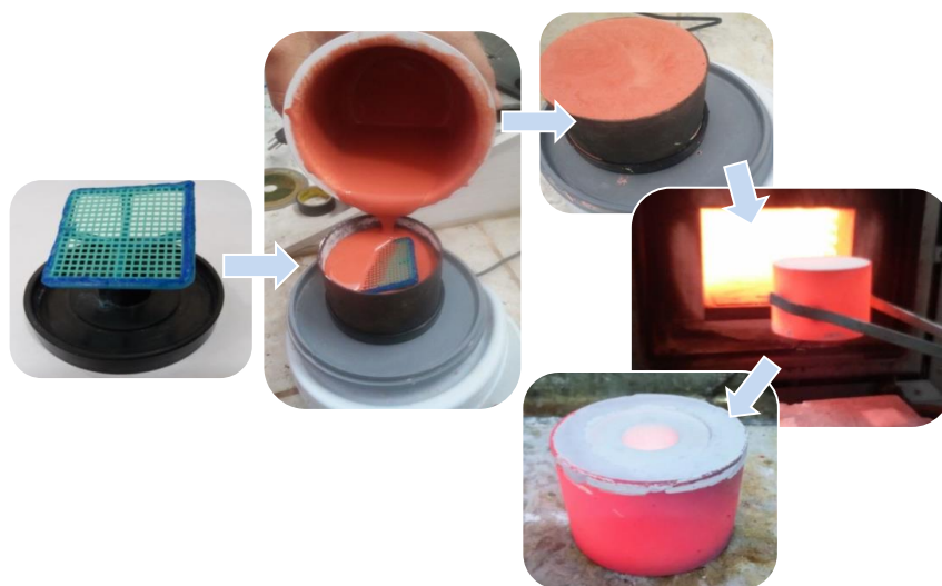
Figure 1. Process sequence for preparation of ceramic molds made through lost-wax.
