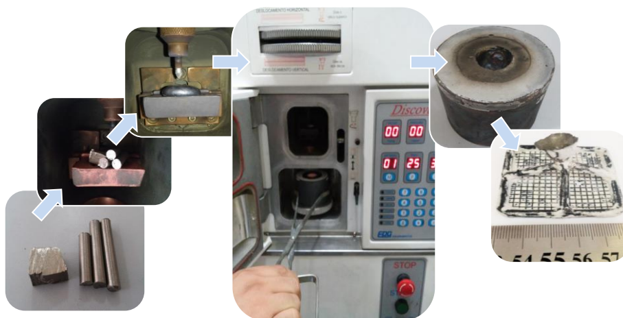
Figure 2. Melting process sequence used for manufacturing of SMA meshes.
