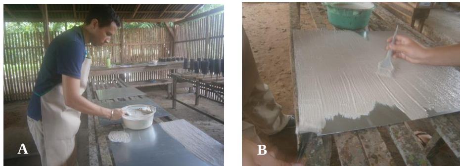
Figure 2. (A) Application of mixed and (B) spreading the mixed latex above the aluminum plate.
