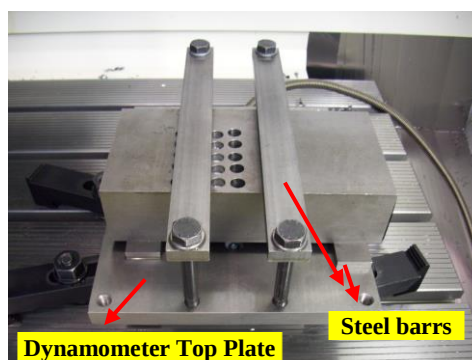
Figure 2. Workpiece set-up on the table of the CNC machine center
