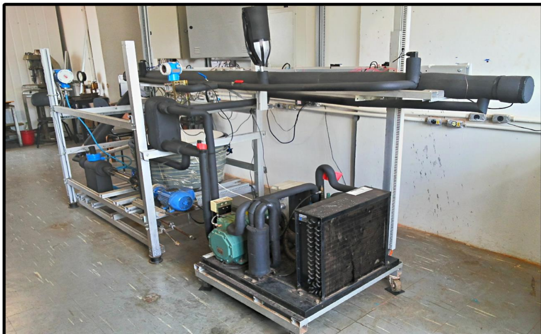
Figure 3. Experimental facility for study of thermo-hydraulic performance of SWCNT nanofluids.
