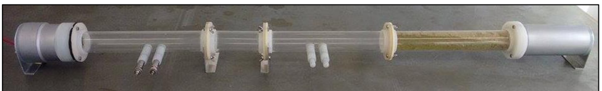
Figure 6. Impedance tube for transmission loss measure.
