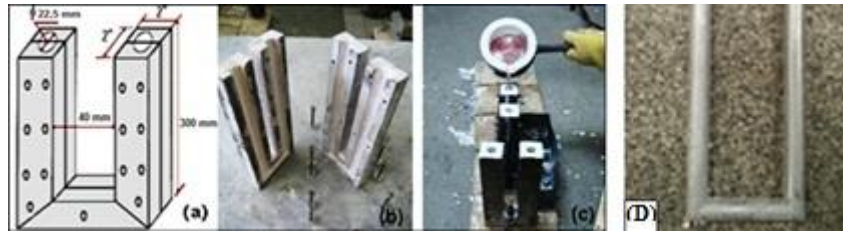
Figure 1 – (a) chill scheme; (b) chill; (c) alloy casting into the crucible used in this process; (D) specimen obtained in the solidification.
