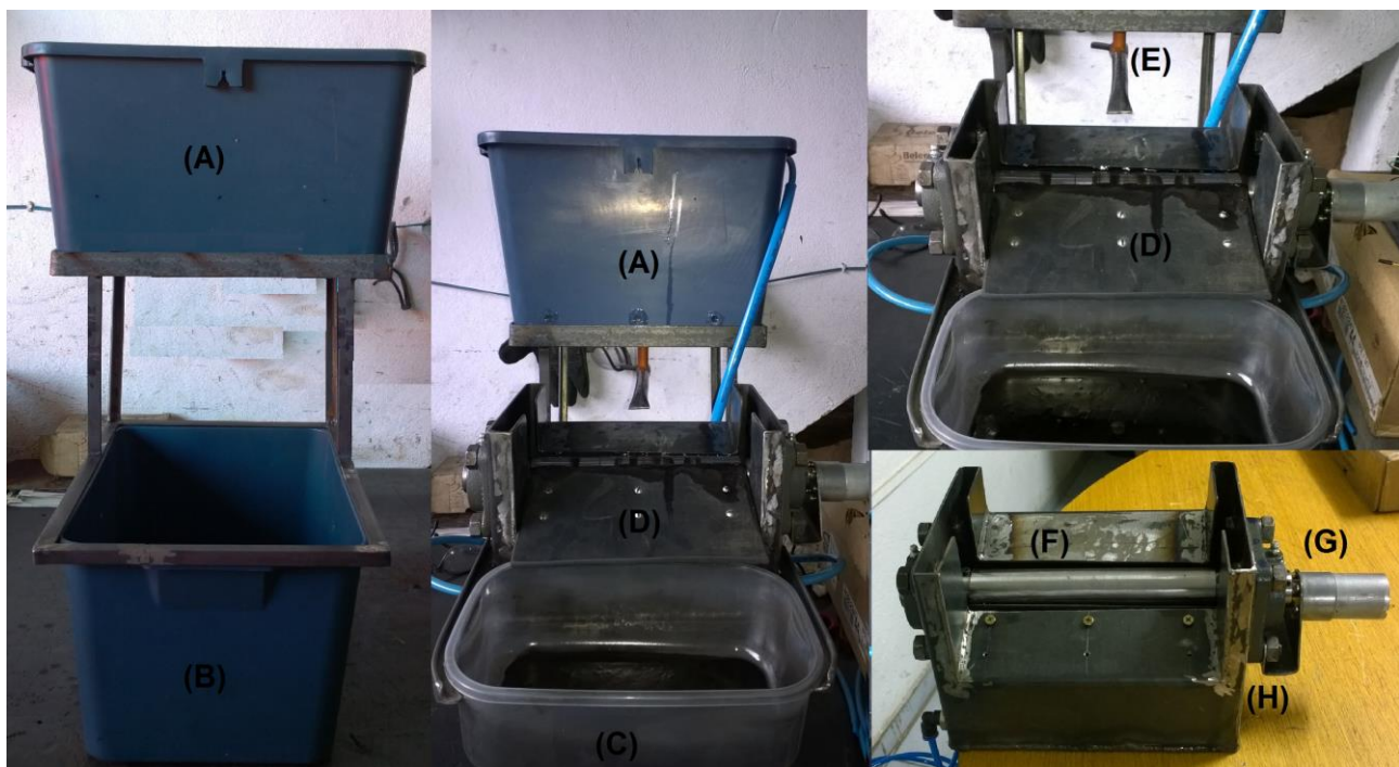
Figure 5. Magnetic filter: (A) Reservoir 1; (B) Reservoir 2; (C) Reservoir 3; (D) Scraper; (E) Tap to feed the filter; (F) Magnetic Roll; (G) Motor – Reducer; (H) Bushing
