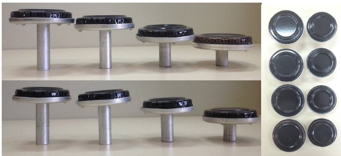
Figure 2. Burners - top and frontal views.
