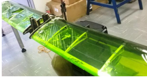
Figure 5. Static test assembly
