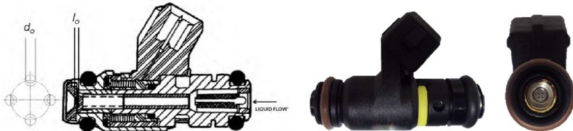
Figure 1. Four-hole port fuel injector used in the tests.
