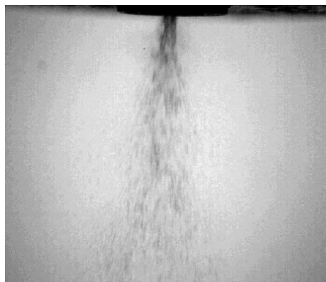
Figure 2. Characteristic image of a fuel injection of the four-hole PFI injector.
