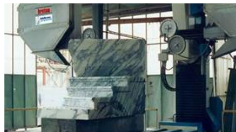
Figure 4. Stationary diamond mono-wire stone cutting 4 axes machine Poker 4 axes by Breton (left) and a helix shaped stone staircase built by it (right) (Breton UK, 2012).
