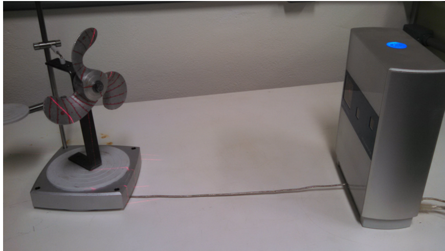
Figure 2. Jet ski rotor under measurement with 3D laser scanner.
