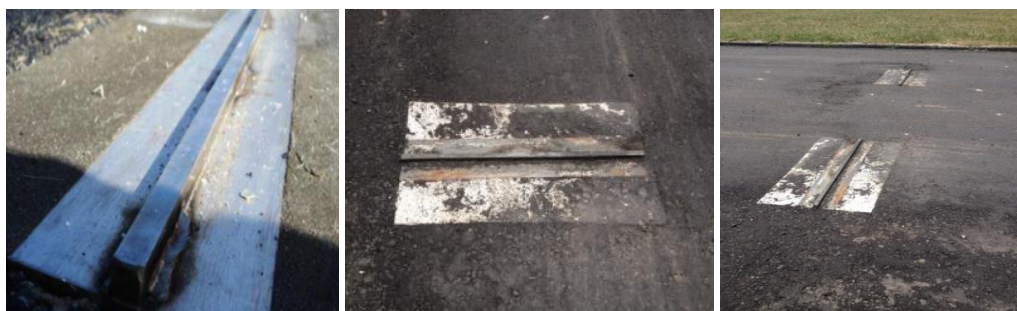
Figure 1. Road obstacles acts as a vertical displacement input to the tires
