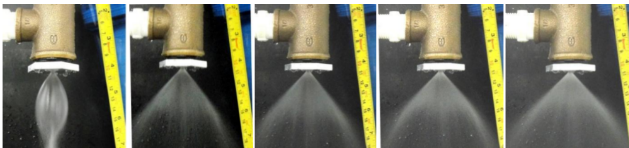
Figure 12. Spray angle at 0,1\text{Bar} , 0,2\text{Bar} , 0,5\text{Bar} , 1\text{Bar} and 2\text{Bar} .
