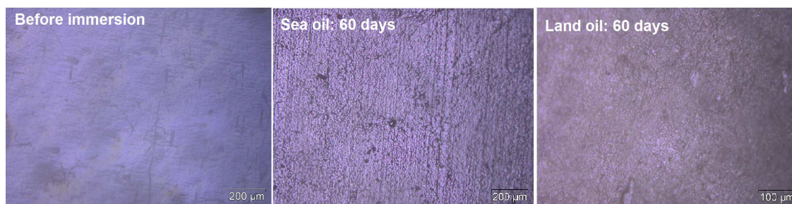
Figure 6. Optical microscopy (x100) of the Sample 01 before immersion and after 60 days of immersion in Sergipe oil from sea and from land
