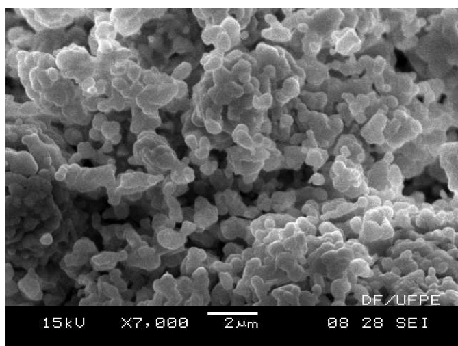
Figure 5. SEM of the Sample 04 (Composite ceramic 78\text{Al}_2\text{O}_3 - 20\text{ZrO}_2 - 2\text{La}_2\text{O}_3 (wt-%))
