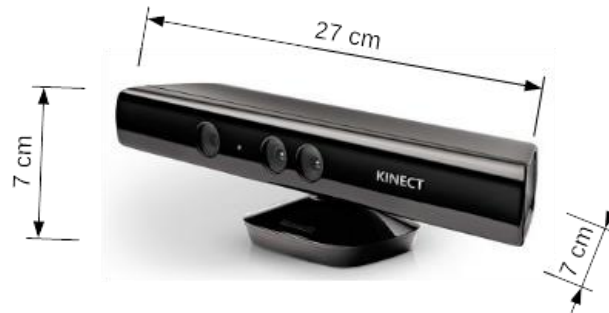
Figure 1. Kinect for Xbox 360 Dimensions
