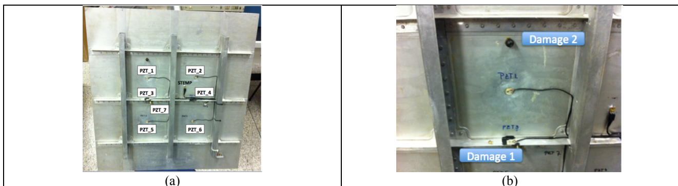
Figure 8. Aeronautical panel instrumented with 7 PZT patches. (a) General view; (b) – Position of simulated damages.
