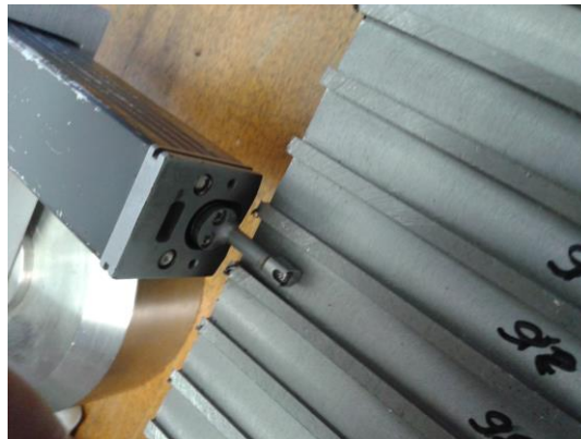
Figure 4. Measurement of the surface roughness at the bottom surface of the channels
