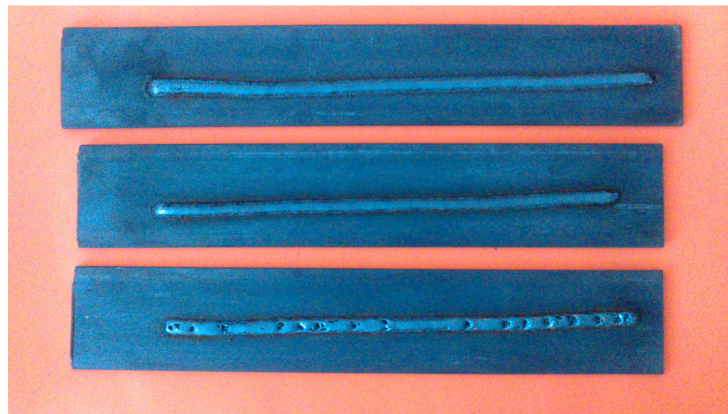
Figure 2. Weld beads for Argon gas flow rates of 16, 8 and 2 L/min (top-down)
