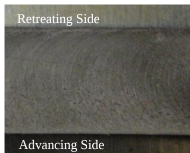
Figure 5. Loss of surface layer at 500 RPM and 65 mm/min
