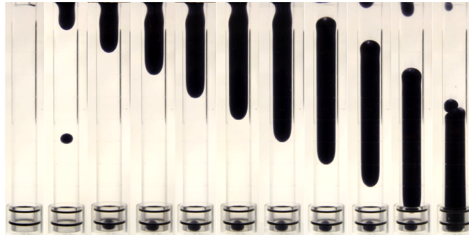
Figure 4. 60% aqueous ethanol solution and soybean oil, positioned with a pump, at 24°C and D = 26 \text{ mm}
