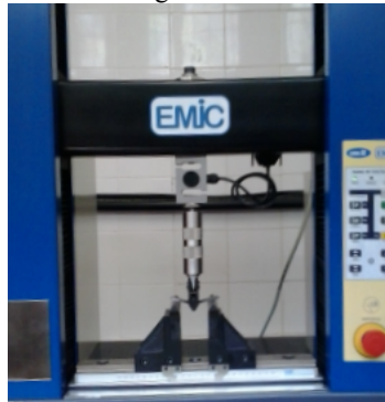
Fig.3 Flexural tests performed in a servo hydraulic Universal testing Machine EMIC Model DL500.
